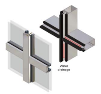
Zone drainage systems feature simple butt jointed mullions and transoms, with each panel acting as an individual unit.
